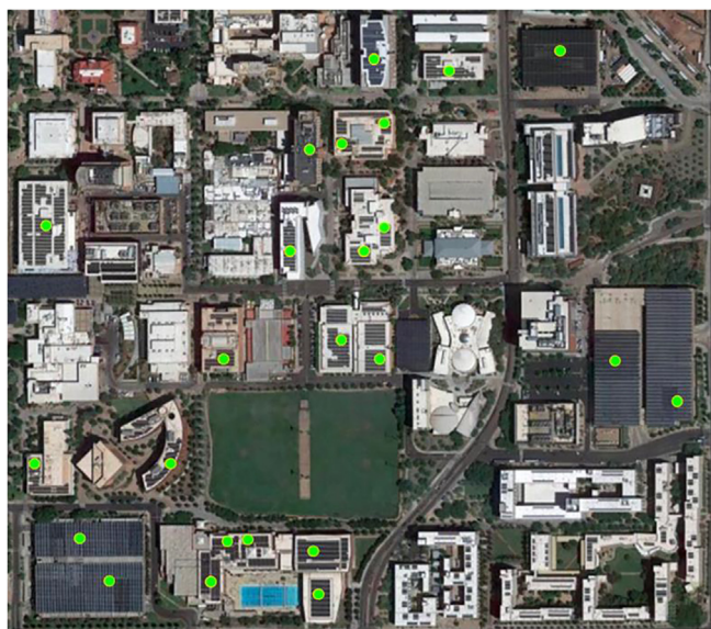
Fig. 1. Photovoltaic systems applied to existing rooftops and parking structures on the campus of Arizona State University, Tempe, Arizona, exemplifying building-applied photovoltaic (BAPV) systems. PV systems are denoted with a green dot. (For interpretation of the references to color in this figure legend, the reader is referred to the web version of this article.)
